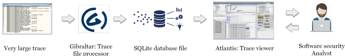
Fig. 1. Before a trace can be inspected by Atlantis, it must be pre-processed offline by Gibraltar. Gibraltar reads the trace and creates a SQLite database that contains the data structures to speed up access to the trace, the memory state delta tree (used for memory reconstruction) and the reconstructed functions and processes.
